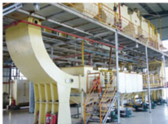
环形浸出器 Loop extractor
